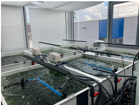
1: The completed large-scale recirculating aquaculture system for seaweed cultivation at TRL6-7. The construction was completed in March and inoculated with Ulva spp. from our shelving unit in April
